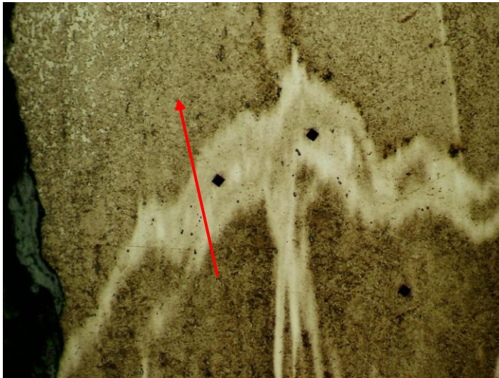
Figure 7.8: Faded yellow white line in knife 323 from Dublin, with some diffusion beyond the weld. Values below the 0.1% detection limit of the SEM-EDS may not be reliable.
