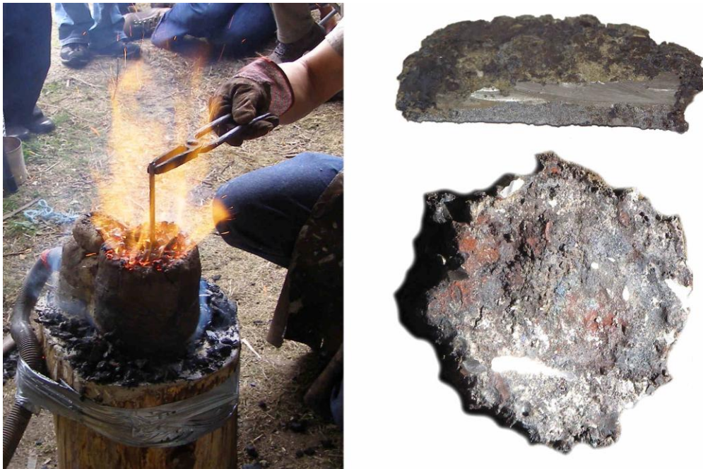
Figure 7.5: Experiment using a small furnace to create liquid steel, demonstrated by Lee Sauder, Shelton Browder and Steve Mankowski based on Ole Evenstad's description in 1790 of a traditional Norwegian steelmaking method (Wagner 1990). This resulted in a small amount of steel which could have been used to edge two or three knives, using the type 2 manufacturing method. Note that the furnace has been placed on a tree trunk resulting in very little evidence for the archaeologist, apart from a bit of vitrified clay.
