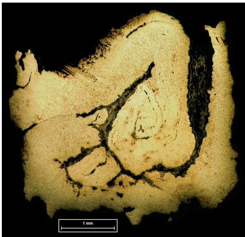
Figure 7.6: Section through bar 60 from Gwithian. Note the folded nature of the knife but also the presence of a white weld line separating two microstructures, this suggests that this bar was originally something else.
