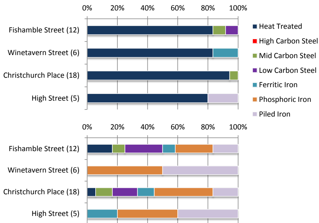
Figure 7.21: Two stacked bar charts showing the alloys used in the cutting edges (top) and knife backs (bottom) in the different areas of Viking Dublin. The raw data is available in table 2.5 in Volume 2.
