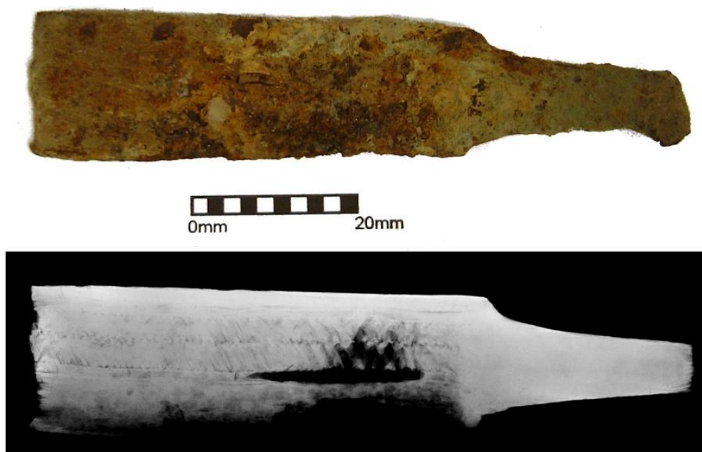
Figure 5.25: Photograph and x-radiograph of pattern-welded knife 2475.
